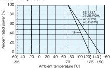
For resistors operated at an ambient temperature of  $70^{\circ}\!\text{C}$  or higher, the power shall be derated in accordance with the above derating curve.
