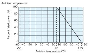
For resistors operated at an ambient temperature of  $70^{\circ}\!\mathrm{C}$  or higher, the power shall be derated in accordance with the above derating curve.
