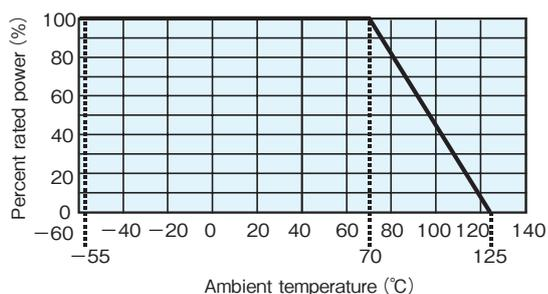
For sensors operated at an ambient temperature of 70°C or higher, the power shall be derated in accordance with the above derating curve.
