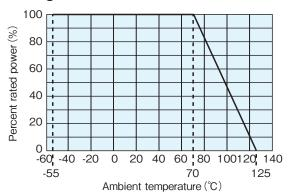
For resistors operated at an ambient temperature of 70°C or higher, the power shall be derated in accordance with derating curve on the left.
